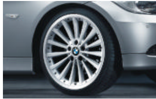
Radial spoke composite wheel 198 19-inch, cast.
